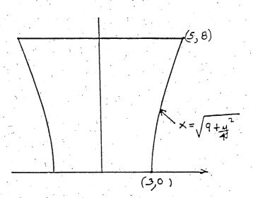
7. A tank which is 9 ft. high, has its base 4 ft. above ground level and is formed by revolving the parabola y = x²/4 + 4 about the y axis. If the tank is filled to a depth of 5 ft. with oil of density 50 lb/ft³, find the work done in pumping all the oil up over the top of the tank.
