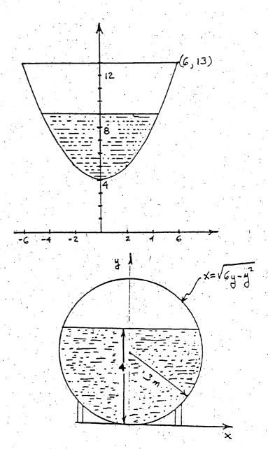
9. An underground storage tank in the shape of a sphere of radius 3 m. is located with its top 6 m. below ground level. The equation for the sphere is x² + y² - 6y = 0 with the origin located at the bottom of the tank. If the tank is filled with gasoline of density ρ = 940 kg/m³ to a depth of 4 m., calculate the work required to pump all the gasoline up to ground level.
